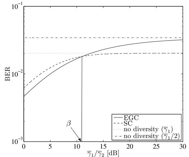
Figure 5: Bit error rate (BER) of selection combining (SC) and equal gain combining (EGC) for BPSK/QPSK with respect to branch unbalance  $\bar{\gamma}_1/\bar{\gamma}_2$  [dB]. Parameter  $\bar{\gamma}_1$  has been set to 5 dB.
