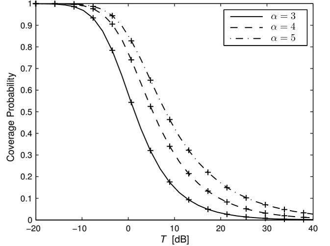
Fig. 1. Coverage probability for different path loss exponents  $\alpha$ . Marks represent simulation results.
