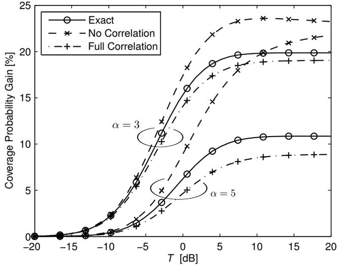
Fig. 5. Coverage probability gain of dual-branch MRC over dual-branch SC for the different correlation models.
