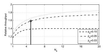
Fig. 6. Performance gain of hopset adaption vs. random hopping for varying intensity of explicit sensing  $N_e$  ( $N=25,\ K=50,\ p_s=0.05$ )
