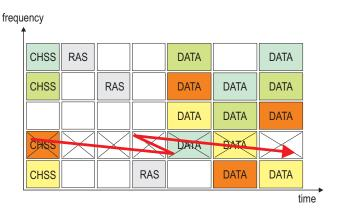
Fig. 2. Frequency hopping scheme with one interfered channel
