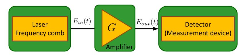
$E_{in}(t) = \sqrt{P_{in}} \sin[\omega t + \phi_0] \qquad \qquad E_{out}(t) = \sqrt{GP_{in}} \sin[\omega t + \phi_0] + N(t)$
