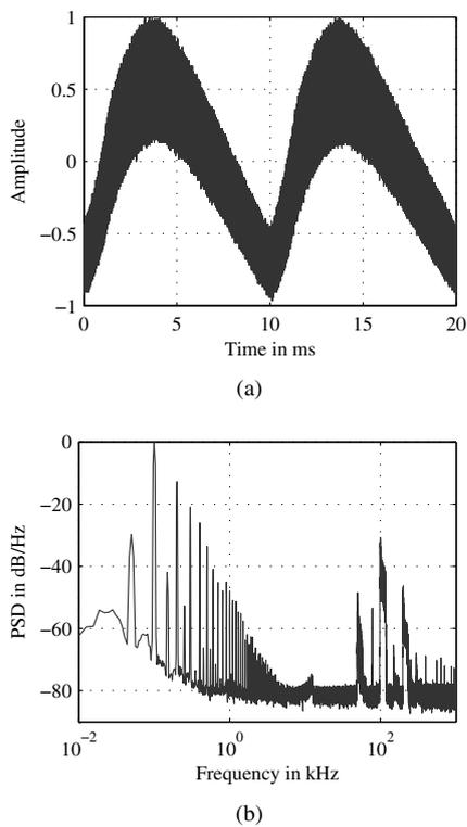
Fig. 2. Compact fluorescent lamp Osram Dulux EL 23 with electronic ballast: (a) Time Waveform (b) Welch Power Spectral Density Estimate
