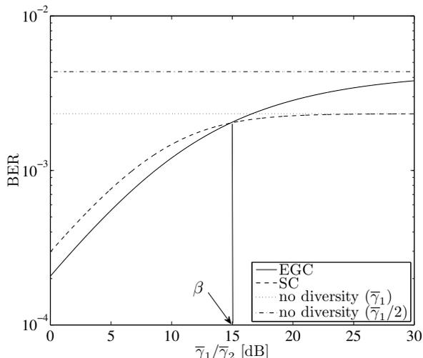
Figure 4: Bit error rate (BER) of selection combining (SC) and equal gain combining (EGC) for BPSK/QPSK with respect to branch unbalance  $\bar{\gamma}_1/\bar{\gamma}_2$  [dB]. Parameter  $\bar{\gamma}_1$  has been set to 10 dB.
