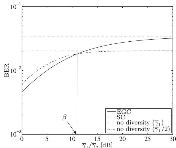
Figure 5: Bit error rate (BER) of selection combining (SC) and equal gain combining (EGC) for BPSK/QPSK with respect to branch unbalance  $\bar{\gamma}_1/\bar{\gamma}_2$  [dB]. Parameter  $\bar{\gamma}_1$  has been set to 5 dB.
