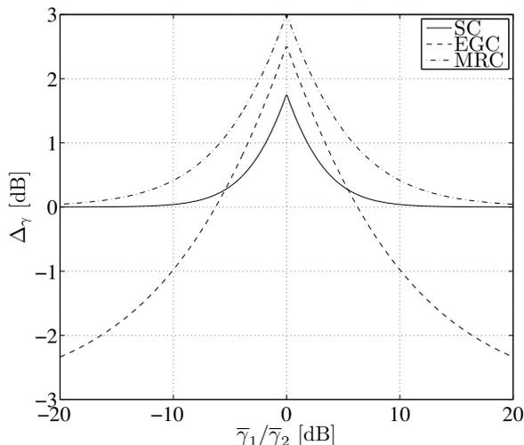
Figure 2: Comparison of the SNR gain  $\Delta_\gamma$  of selection combining (SC), equal gain combining (EGC) and maximal ratio combining (MRC) with respect to branch unbalance  $\bar{\gamma}_1/\bar{\gamma}_2$  [dB].
