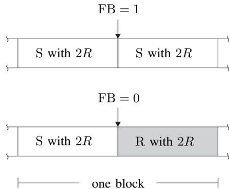
Fig. 2. Transmission model for incremental relaying. If the source-destination link is not in outage (feedback  $\text{FB} = 1$ ), the source transmits during the second sub-block, too. If the source-destination link is in outage (feedback  $\text{FB} = 0$ ), the relay aids communication during the second sub-block.
