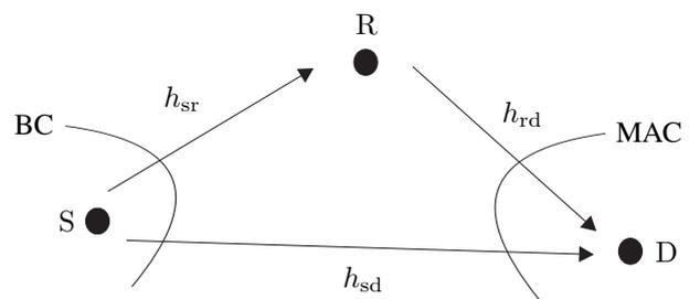
Fig. 1. Network consisting of source S, relay R, and destination D. Channel gains are represented by  $h_{sd}$ ,  $h_{sr}$ , and  $h_{rd}$ . BC and MAC denote the cuts for the broadcast channel and the multiple access channel, respectively.
