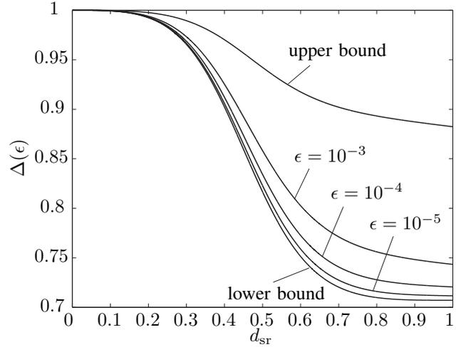
Fig. 4. Ratio  $\Delta(\epsilon)$  of  $\epsilon$ -outage capacity of incremental relaying to the cut-set bound for  $\gamma \rightarrow 0$  and  $\alpha = 3$ . When the relay is placed close to the destination, we get  $\Delta(\epsilon) = 1/\sqrt{2}$ . When the relay is located close to the source, we have  $\Delta(\epsilon) = 1$ .
