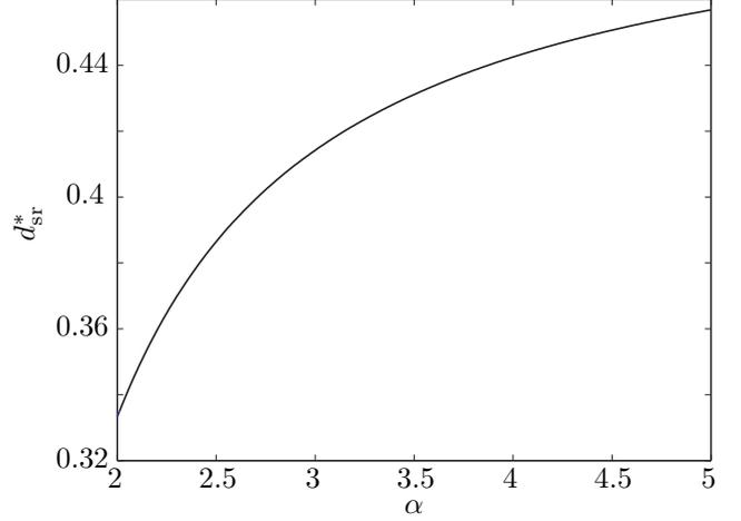
Fig. 3. Optimal source-relay distance  $d_{\text{sr}}^*$  versus path-loss factor  $\alpha$ . For  $\alpha \rightarrow \infty$   $d_{\text{sr}}^*$  tends asymptotically to  $d_{\text{sr}}^* = 0.5$ .  $d_{\text{sr}}^*(\alpha = 2) = 1/3$ .
