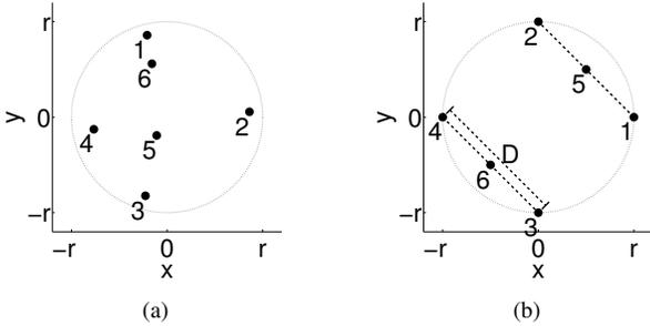
Fig. 1. a) Network with arbitrarily distributed nodes,  $r = 1000$  m,  $\alpha = 4$ ,  $P = 0.1$  W,  $W = 20$  MHz,  $T = 293$  K,  $\eta \approx 4 \cdot 10^{-21}$  W. b) Circular network topology for testing the parameter dependency of the transmission rates.
