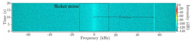
(a) Received PT signal with DC offset at  $f_{\text{LOOffset}} = 55$  kHz and flicker noise ( $1/f$  noise)
