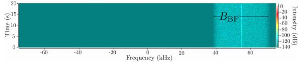
(b) Signal after band pass filtering ( $B_{\text{BF}} = 30$  KHz) at  $f_{\text{LOOffset}}$
