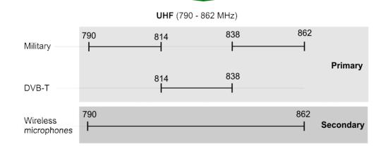
Example: Current assignment of frequencies between 790 MHz and 862 MHz ("Digital Dividend")
